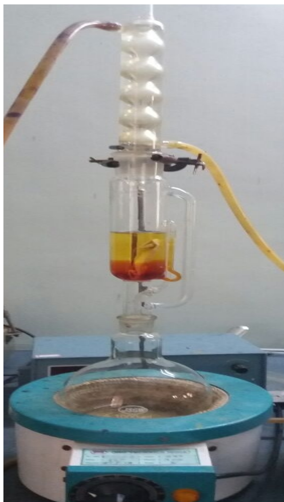
Figure 2: Soxhlet extraction of Capsaicinoid from chili samples
